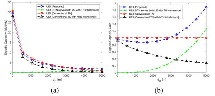
Fig. 2: (a) Ergodic capacity and (b) ergodic capacity gain of UE1 with respect to the distance between UE1 and TN BS.
