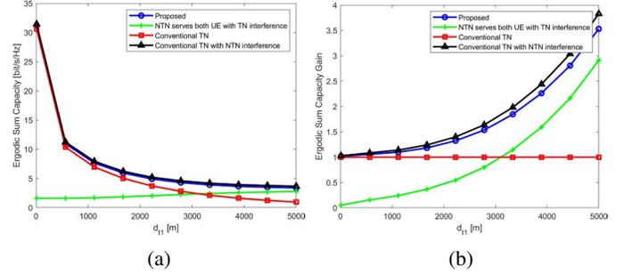
Fig. 3: (a) Ergodic sum capacity and (b) ergodic sum capacity gain of HSTN with respect to the distance between UE1 and TN BS.
