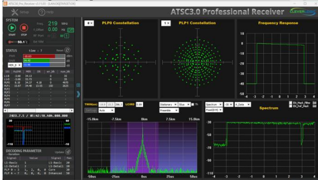
Fig. 7. Remodulated ATSC 3.0 UHD output of iMATV
