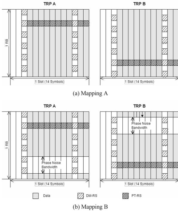
Fig. 4. Examples of RS mapping for downlink multi-TRP scenario
