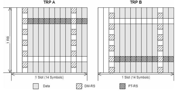
Fig. 2. Conventional resource mapping for downlink multi-TRP scenario
