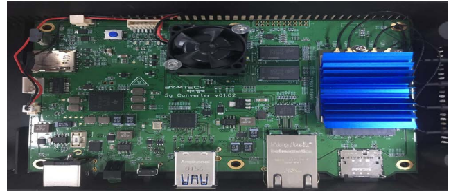
Fig. 2. Hardware built for the 5G-communication-based data transmission system.
