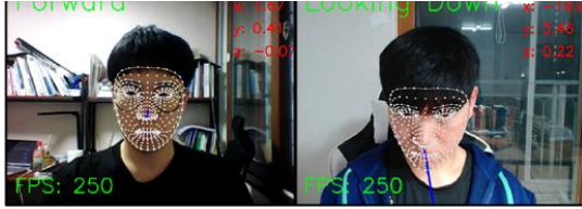
Fig. 1. Exmpales of viewing images captured in the online performance environment. The white face mesh points are the result of using the face landmark detection algorithm (mediapipe[8]) to estimate the 3D face pose.
