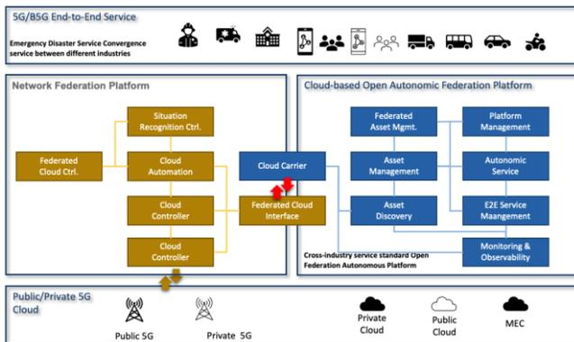
Figure 5. CloudMesh<sup>I5S</sup> PoC Implementation Architecture
