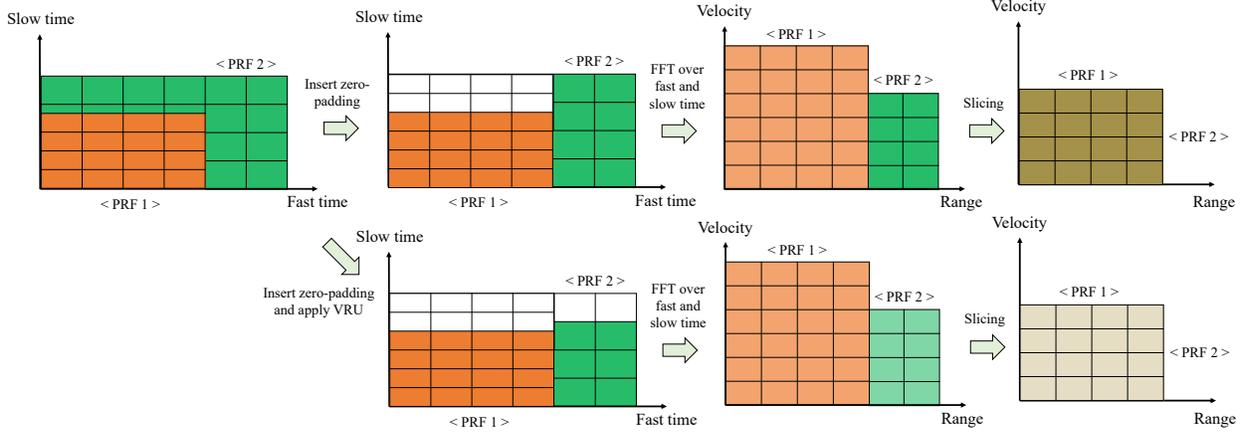
Fig. 2: Process of velocity resolution uniformization and RD map slicing for multiple PRF radar data
