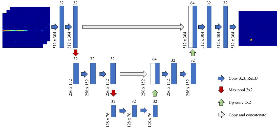
Fig. 4: U-Net architecture for sea clutter suppression and target detection in RD maps
