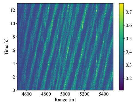
Fig. 1: Range-time intensity map showing sea clutter patterns in radar signals
